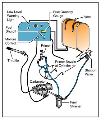
Figure 5-9. A typical gravity feed fuel system, in a helicopter with a reciprocating engine, contains the components shown here.
