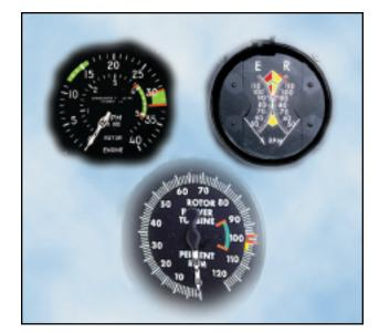
Figure 5-3. There are various types of dual-needle tachometers, however, when the needles are superimposed or married, the ratio of the engine r.p.m. is the same as the gear reduction ratio.
