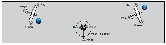
Figure 13-5. By interpreting the position lights on other aircraft, you can determine whether the aircraft is flying away from you or is on a collision course. If you see a red position light to the right of a green light, such as shown by aircraft number 1, it is flying toward you. You should watch this aircraft closely and be ready to change course. Aircraft number 2, on the other hand, is flying away from you, as indicated by the white position light.
