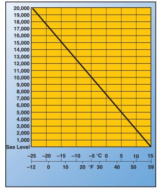
Figure 20-6. Standard temperature chart.
