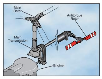
Figure 1-6. Typically, the engine drives the main rotor through a transmission and belt drive or centrifugal clutch system. The antitorque rotor is driven from the transmission.
