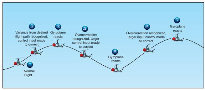
Figure 21-1. Pilot-induced oscillation can result if the gyroplane's reactions to control inputs are not anticipated and become out of phase.
