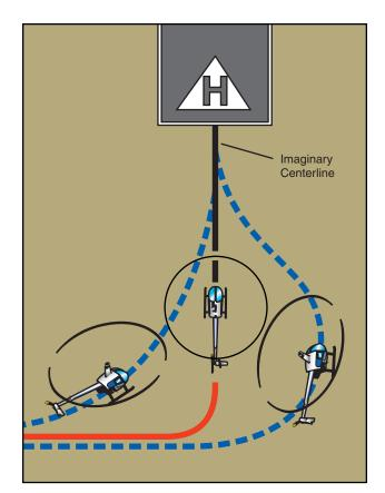
Figure 9-19. Plan the turn to final so the helicopter rolls out on an imaginary extension of the centerline for the final approach path. This path should neither angle to the landing area, as shown by the helicopter on the left, nor require an S-turn, as shown by the helicopter on the right.
