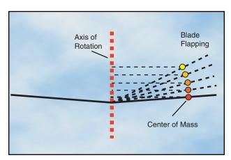
Figure 3-5. The tendency of a rotor blade to increase or decrease its velocity in its plane of rotation due to mass movement is known as Coriolis Effect, named for the mathematician who made studies of forces generated by radial movements of mass on a rotating disc.
