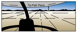
Figure 9-11. You can maintain a straight-and-level attitude by keeping the tip-path plane parallel to and a constant distance above or below the natural horizon. For any given airspeed, this distance remains the same as long as you sit in the same position in the same type of aircraft.
