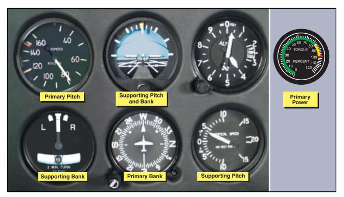
Figure 12-18. Flight instrument indications in a stabilized, constant airspeed climb.
