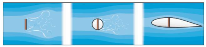
Figure 2-12. It is easy to visualize the creation of form drag by examining the airflow around a flat plate. Streamlining decreases form drag by reducing the airflow separation.
