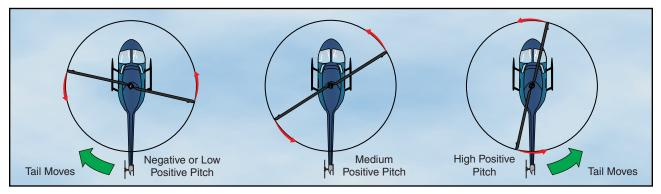
Figure 4-6. Tail rotor pitch angle and thrust in relation to pedal positions during cruising flight.
