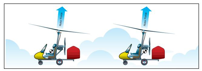
Figure 16-10. If the CG is located in front of the rotor force line, the gyroplane is more stable than if the CG is located behind the rotor force line.
