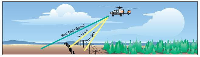
Figure 21-3. Any deviation from best glide speed will reduce the distance you can glide and may cause you to land short of a safe touchdown point.
