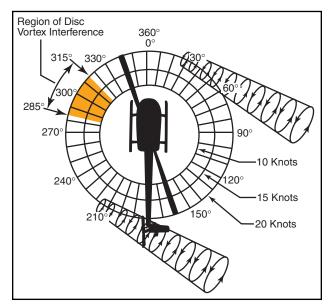
Figure 11-10. Main rotor disc vortex interference.
