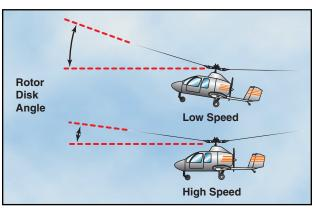
Figure 20-7. The angle of the rotor disc decreases at higher cruise speeds, which increases pitch control sensitivity.
