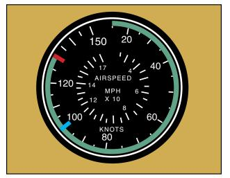
Figure 6-2. Typical airspeed indicator limitations and markings.
