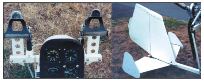
Figure 17-3. Foot pedals provide rudder control and operation is similar to that of an airplane.
