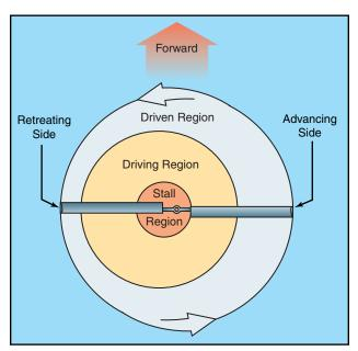
Figure 16-5. Rotor disc regions in forward autorotative flight.
