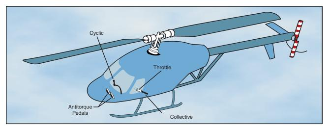
Figure 1-7. Location of flight controls.
