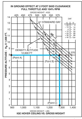
Figure 8-2. In Ground Effect Hover Ceiling versus Gross Weight Chart.
