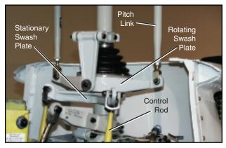
Figure 5-8. Collective and cyclic control inputs are transmitted to the stationary swash plate by control rods causing it to tilt or to slide vertically. The pitch links attached from the rotating swash plate to the pitch horns on the rotor hub transmit these movements to the blades.
