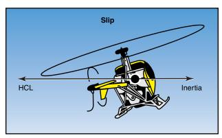
Figure 9-13. During a slip, the rate of turn is too slow for the angle of bank used, and the horizontal component of lift (HCL) exceeds inertia.
