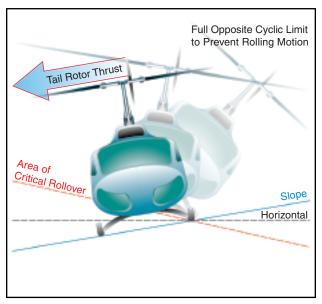
Figure 11-8. Downslope rolling motion.
