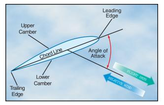
Figure 2-3. Aerodynamic terms of an airfoil.
