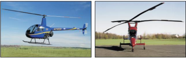
Figure 1-2. Helicopters can have a single main rotor or a dual rotor system.
