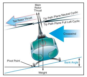
Figure 11-6. Forces acting on a helicopter with right skid on the ground.
