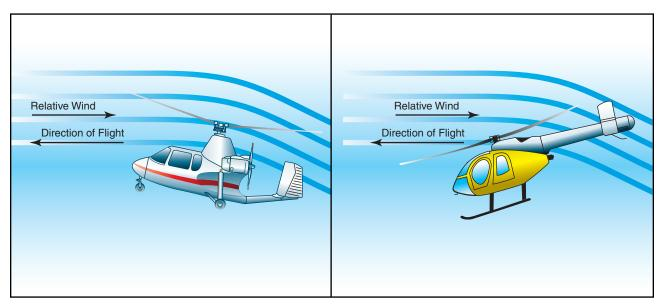
Figure 16-1. Airflow through the rotor system on a gyroplane is reversed from that on a powered helicopter. This airflow is the medium through which power is transferred from the gyroplane engine to the rotor system to keep it rotating.
