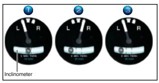
Figure 12-8. In a coordinated turn (instrument 1), the ball is centered. In a skid (instrument 2), the rate of turn is too great for the angle of bank, and the ball moves to the outside of the turn. Conversely, in a slip (instrument 3), the rate of turn is too small for the angle of bank, and the ball moves to the inside of the turn.
