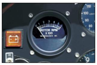
Figure 18-6. A rotor tachometer can be very useful to determine when rotor r.p.m. is sufficient for takeoff.
