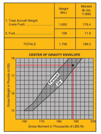
Figure 19-4. Center of gravity envelope chart.
