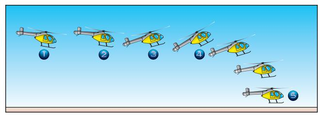
Figure 10-3. Rapid deceleration or quick stop.
