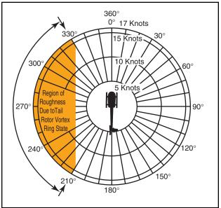
Figure 11-12. Tail rotor vortex ring state.
