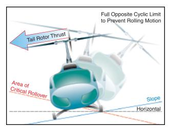
Figure 11-7. Upslope rolling motion.
