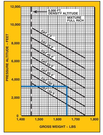
Figure 6-7. One of the performance charts in the Performance Section is the "In Ground Effect Hover Ceiling versus Gross Weight" chart. This chart allows you to determine how much weight you can carry and still operate at a specific pressure altitude, or if you are carrying a specific weight, what is your altitude limitation.
