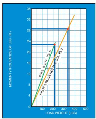
Figure 7-7. Moments for fuel, pilot, and passenger.
