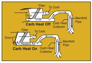
Figure 5-11. When you turn the carburetor heat ON, normal air flow is blocked, and heated air from an alternate source flows through the filter to the carburetor.
